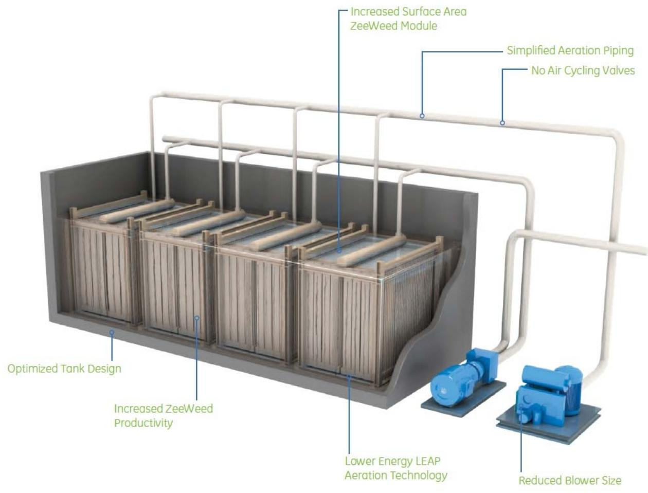
**ILLUSTRATION OF A SUBMERGED MEMBRANE FILTER (GENERAL ELECTRIC)**
