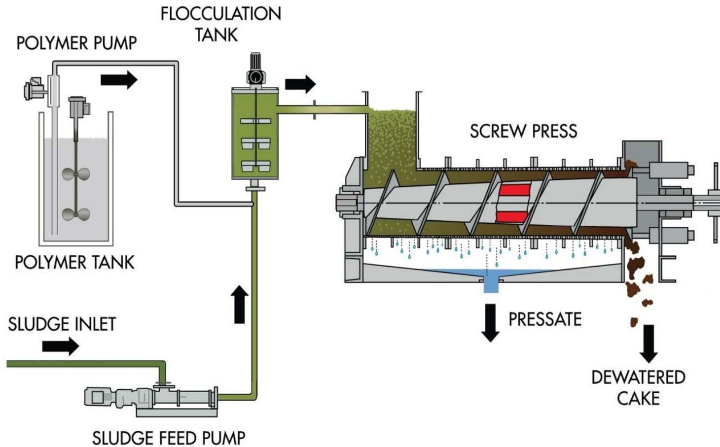
**SCHEMATIC OF A SCREW PRESS (FKC CO.)**
