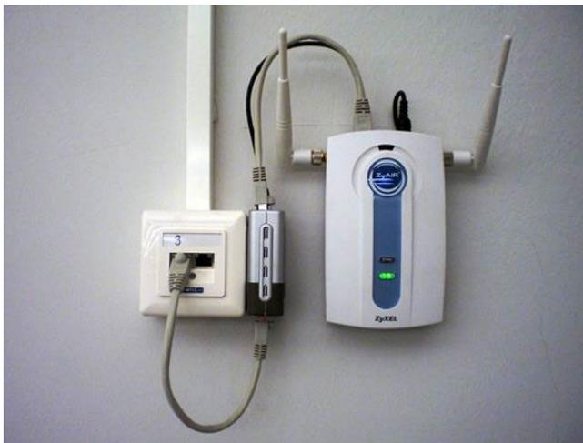
Given a single Power over Ethernet connection (single gray cable looping below), a PoE splitter provides both data (gray cable looping above) and power (black cable also looping above) connections for a wireless access point. The splitter is the silver and black box in the middle, between the wiring box on the left and the access point (with its two antennas) on the right. The PoE connection eliminates the need for a nearby power outlet.
