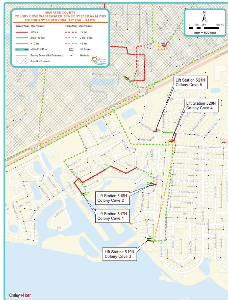
Figure 8: Existing System Modeled Velocities and Flow Capacities
