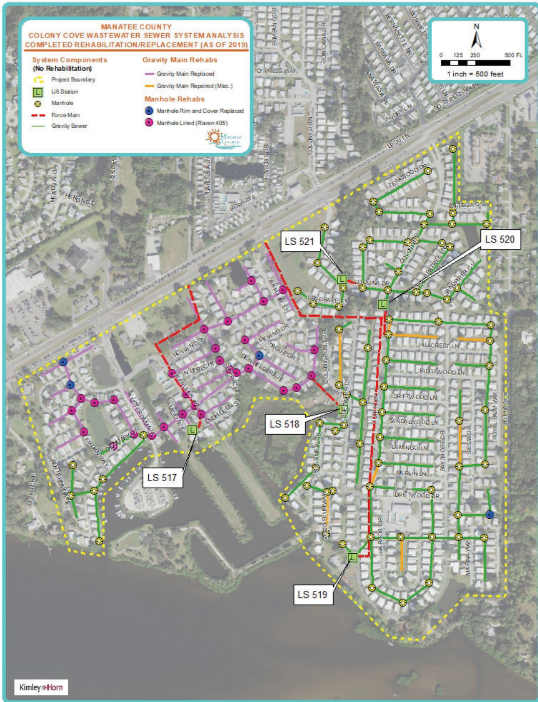
Figure 1: Existing Sewer System with Rehabilitation and Replacements
