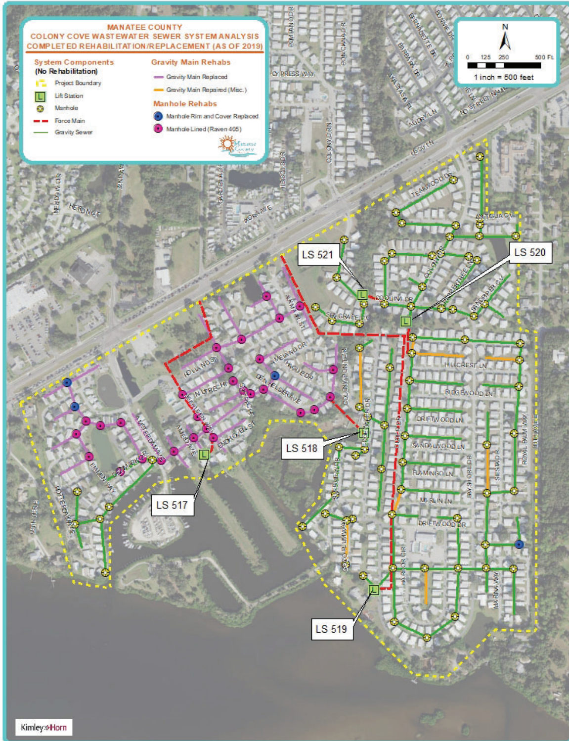
Figure 1 Existing Sewer System with Rehabilitation and Replacements
