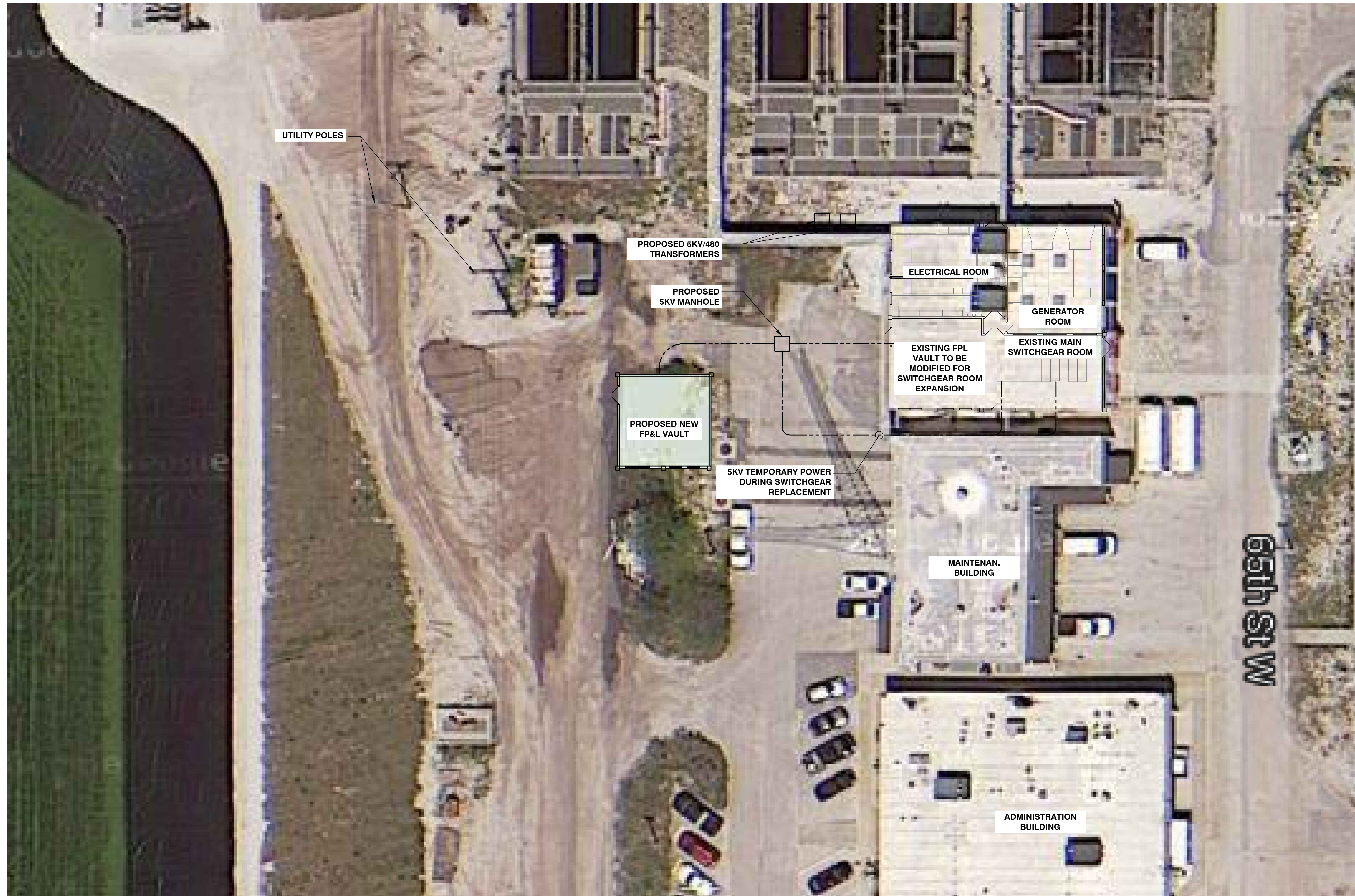
FIGURE No. 7 PROPOSED FP&L VAULT AND SWITCHGEAR LOCATION
