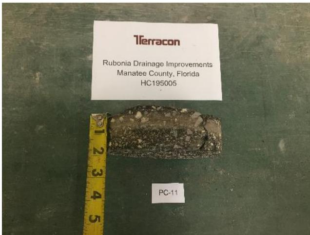
Core PC-11, 1 3/4" Asphalt (Full-Depth Crack)
