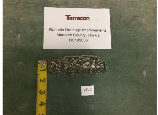
Core PC-2, 1" Asphalt (Full-Depth Crack)
