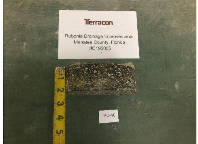
Core PC-10, 2" Asphalt (Full-Depth Crack)
