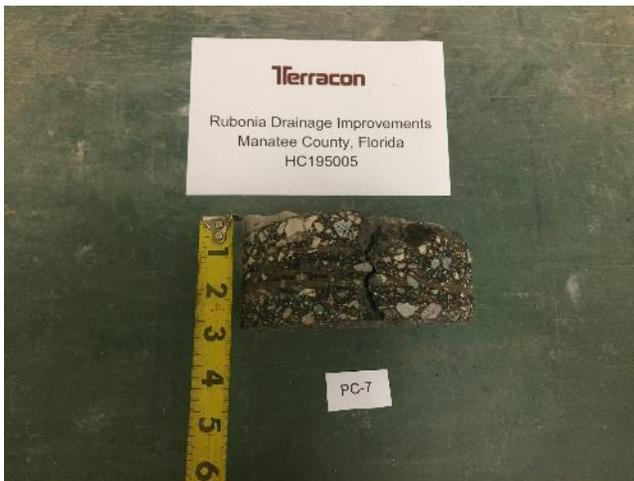
Core PC-7, 2 1/4" Asphalt (Full-Depth Crack)
