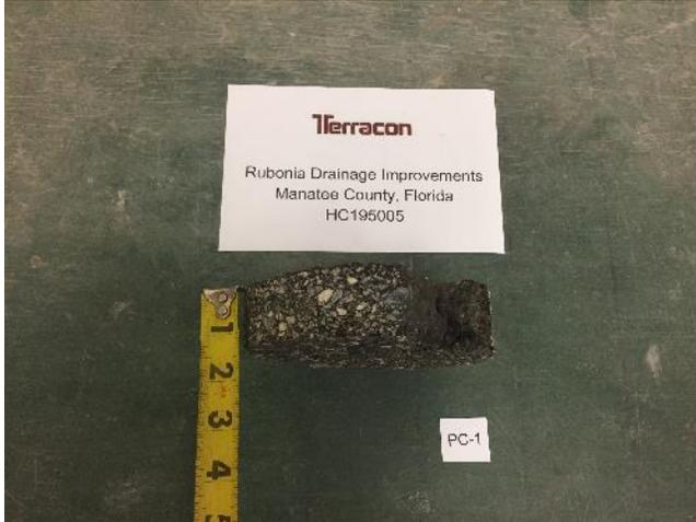
Core PC-1, 1 1/4" Asphalt (Full-Depth Crack)
