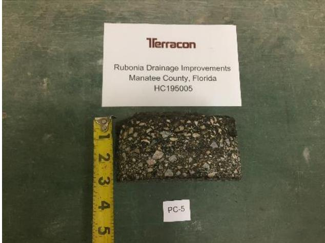
Core PC-5, 3" Asphalt (Full-Depth Crack)
