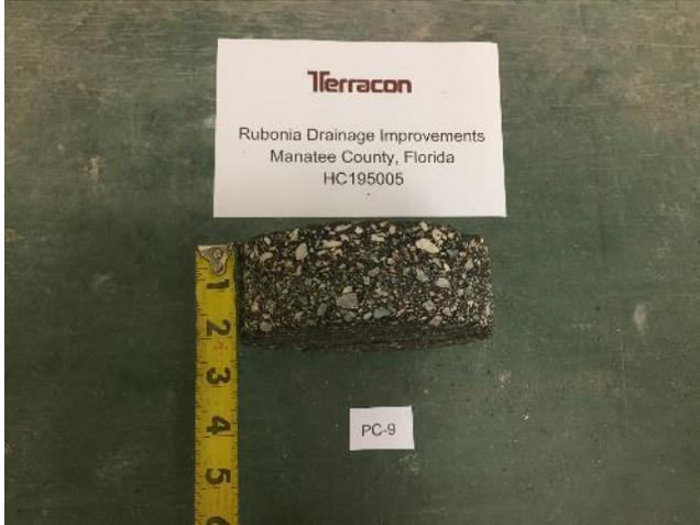
Core PC-9, 2" Asphalt (Full-Depth Crack)
