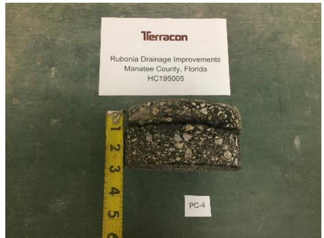
Core PC-4, 2 3/4" Asphalt (Full-Depth Crack)
