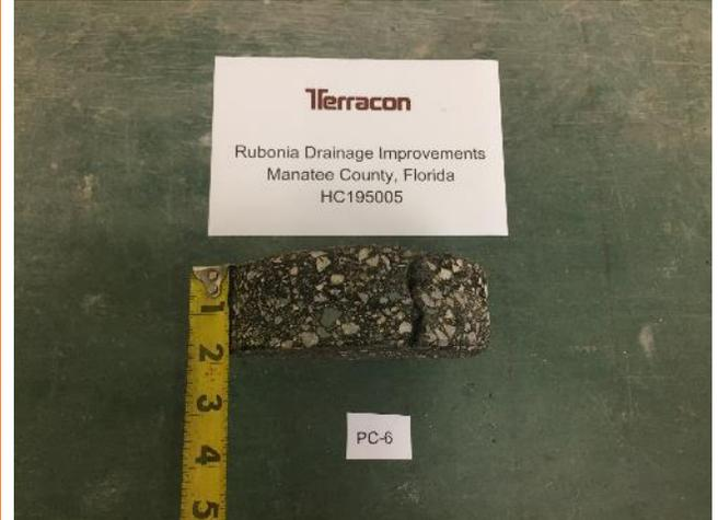
Core PC-6, 1 3/4" Asphalt (Full-Depth Crack)
