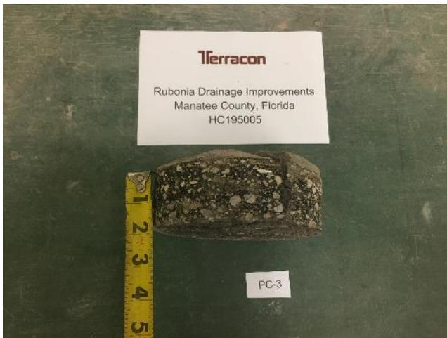
Core PC-3, 2" Asphalt (Full-Depth Crack)
