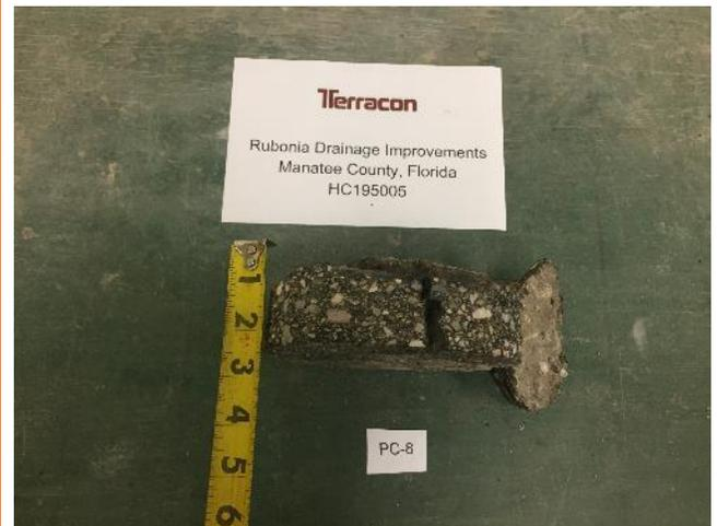
Core PC-8, 2 1/4" Asphalt (Full-Depth Crack)
