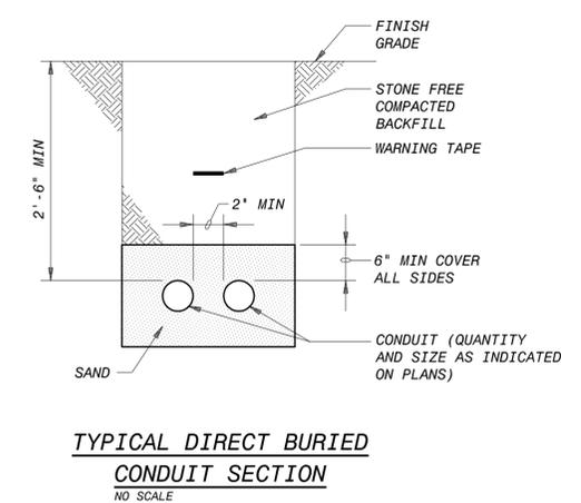
**TYPICAL DIRECT BURIED CONDUIT SECTION**
