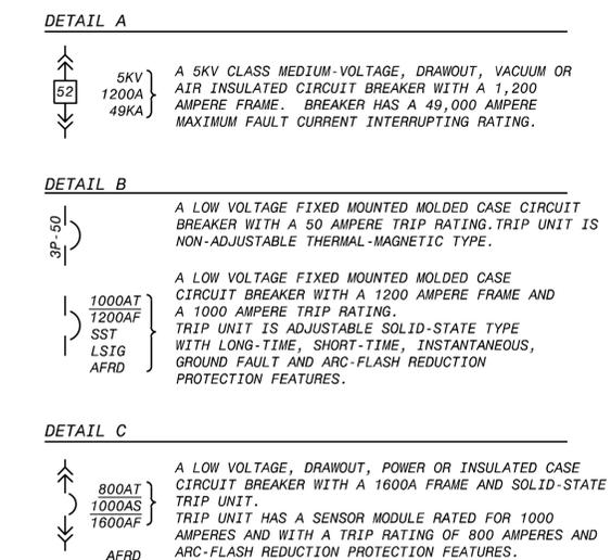
**CONDUIT & WIRING INSTALLATION LEGEND**
