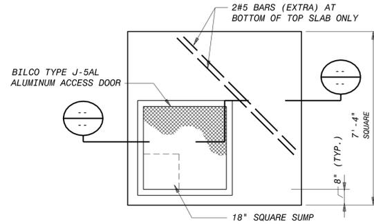
**TYPICAL ELECTRICAL MANHOLE (SINGLE CHAMBER)**
