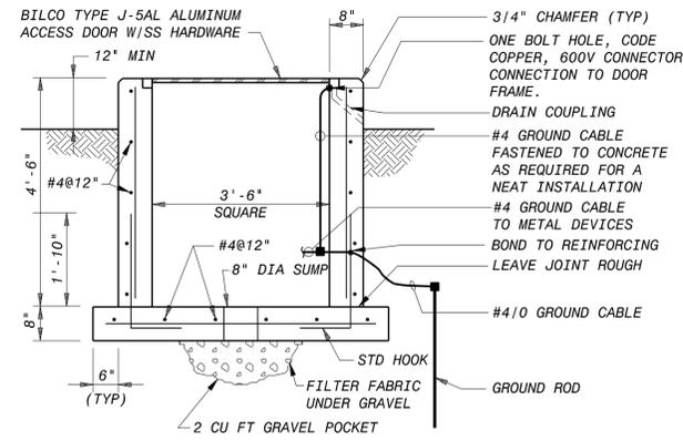
**TYPICAL ELECTRICAL HANDHOLE DETAIL**
