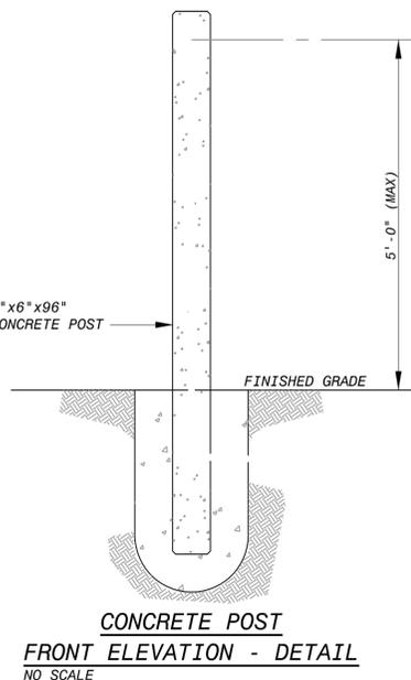
**CONCRETE POST FRONT ELEVATION - DETAIL**
