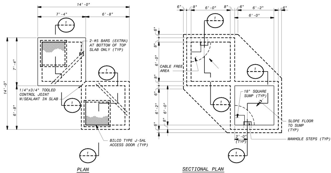
**ELECTRICAL MANHOLE (DOUBLE CHAMBER)**
