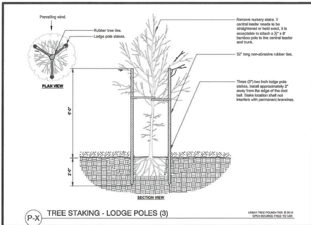
Figure 1 - Tree Staking Example
