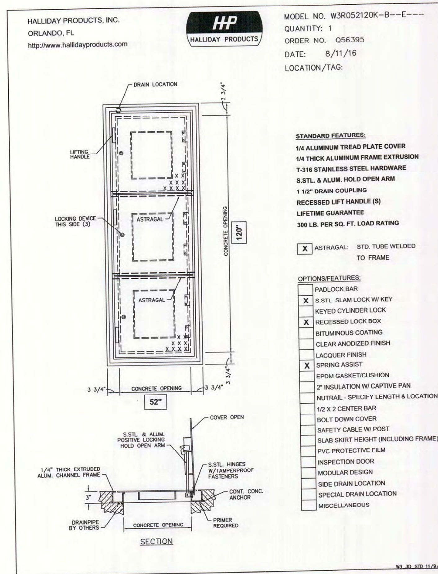
ACCESS HATCH DETAIL
