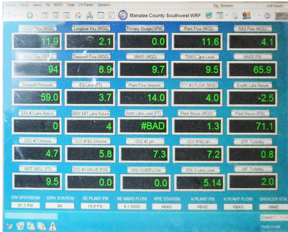
**C CONTROL CENTER - SCADA SCREEN** SCALE: - FILE: -
