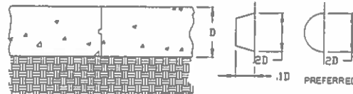
TYPE 'C' CONSTRUCTION JOINT NTS
