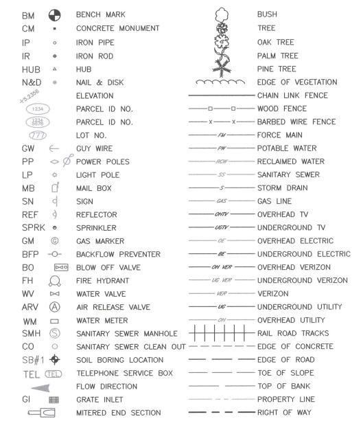
RIGHT OF WAY CONCRETE CONC **ASPHALT** DRIVEWAY SWK SIDEWALK EDGE OF PAVEMENT BACK OF CURB BOC
