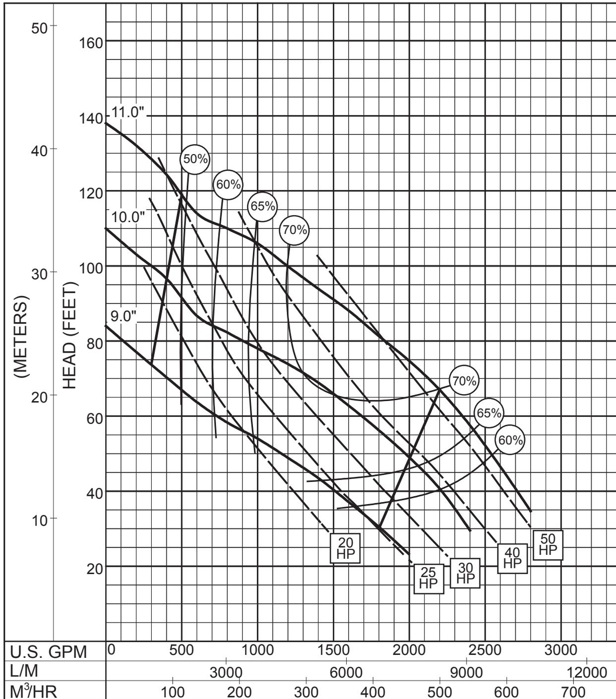
The curves reflect maximum performance characteristics without exceeding full load (Nameplate) horsepower. All pumps have a service factor of 1.2. Operation is recommended in the bounded area with operational point within the curve limit. Performance curves are based on actual tests with clear water at 70° F. and 1280 feet site elevation.
