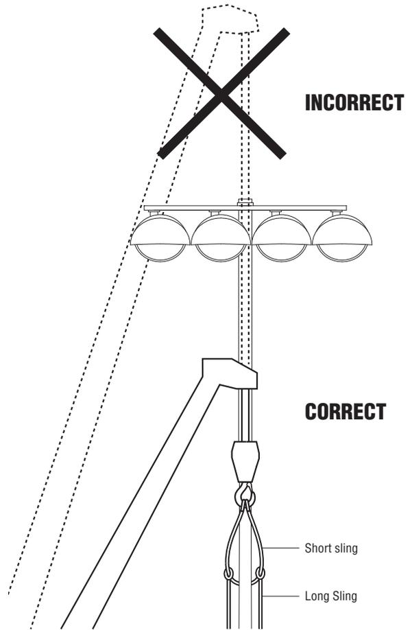
**8** When pole is suspended, insert rotator bar to clamp and turn to lock in place. Guide pole into position over base using rotator bar and lower onto base. Do not allow pole to seat on base until it is properly aimed (step 9). Pole should rotate with reasonable force applied to bar, but not freely.
