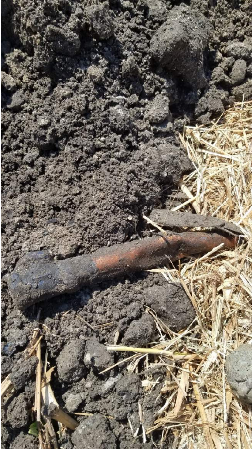
Photograph 7. Test Pit TP-6 metal pipe encountered.
