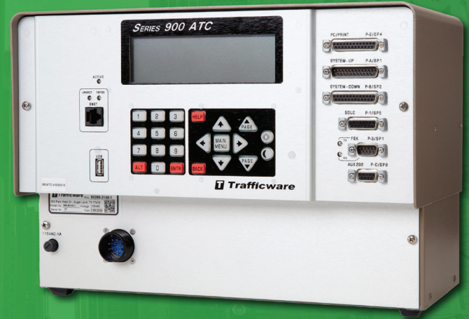
Pictured above: 980 ATC Type 1 Controller with Ethernet & USB
