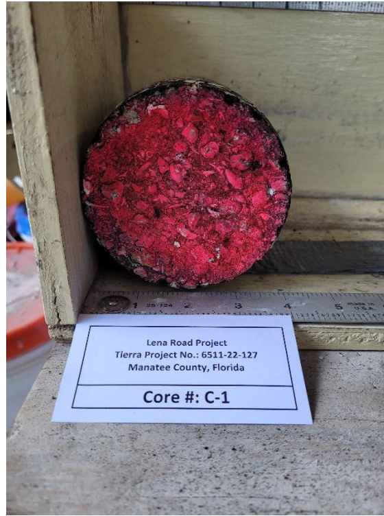
Photograph 2. Pavement Core No. C-1 Top View
