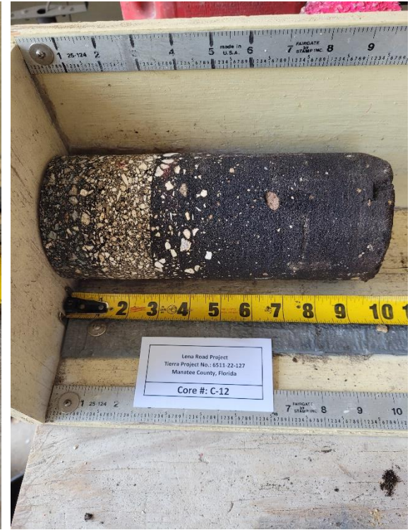
Photograph 36. Pavement Core No. C-12 Side View
