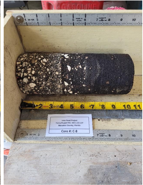
Photograph 24. Pavement Core No. C-8 Side View
