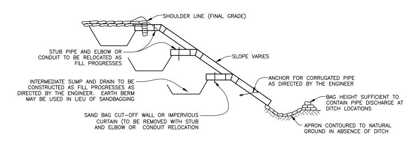
SECTION AA TEMPORARY SLOPE DRAIN
