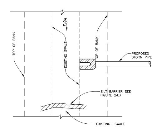
SILT BARRIER AT CONNECTION OF STORM PIPE TO EXISTING SWALE
