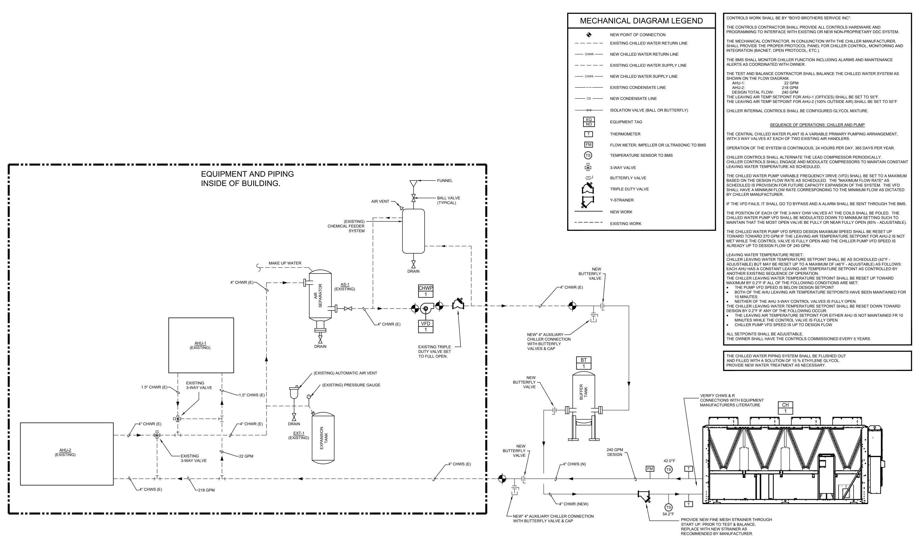
MECHANICAL CHILLED WATER FLOW & PIPING DIAGRAM
