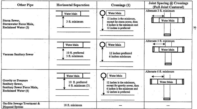
(1) Water main should cross above other pipe. When water main must be below other pipe, the minimum separation is 12 inches.
