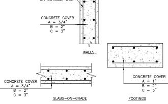
A = NO EXPOSURE TO GROUND OR WEATHER AFTER FORM REMOVAL. B = EXPOSURE TO GROUND OR WEATHER AFTER FORM REMOVAL C = CONCRETE PLACED AGAINST GROUND.
