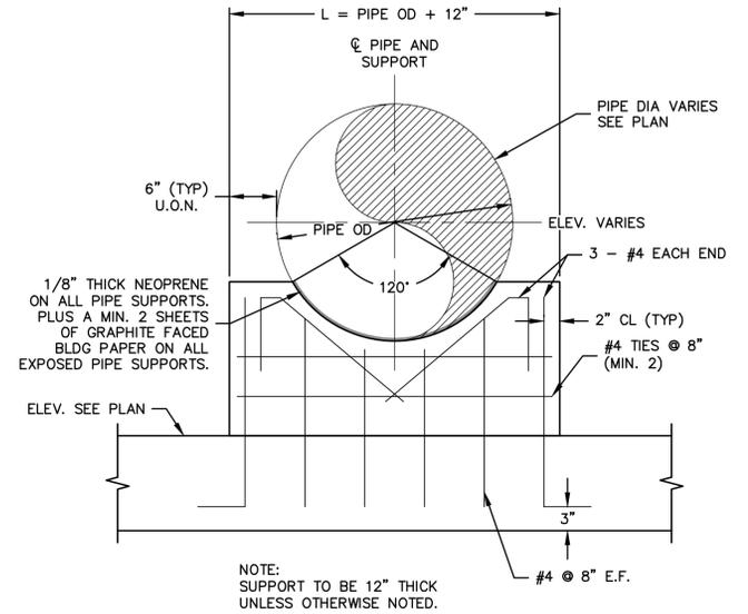
8- DETAIL - TYP. PIPE SUPPORT DETAIL
