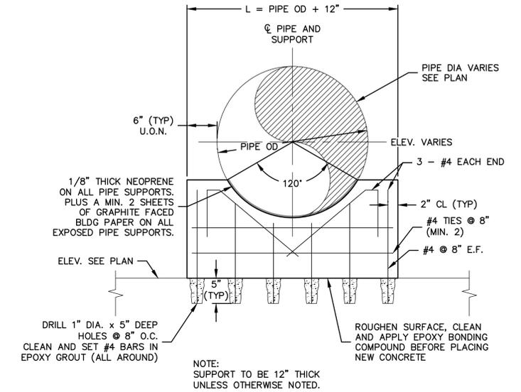
9- DETAIL - TYP. PIPE SUPPORT DETAIL ON EXISTING CONCRETE
