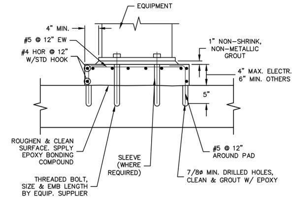
7- DETAIL - TYP. EQUIPMENT SUPPORT PAD ON EXISTING CONCRETE
