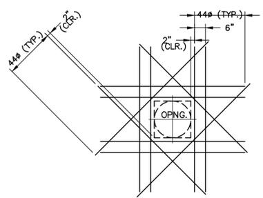
2 - DETAIL-TYP. REINF. @ SLAB / WALL OPNG
