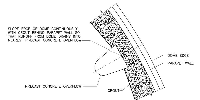
PARAPET WALL PLAN W/OVERFLOW
