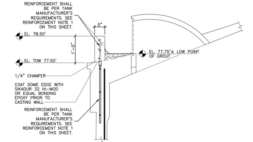
PARAPET WALL DETAIL W/OVERFLOW
