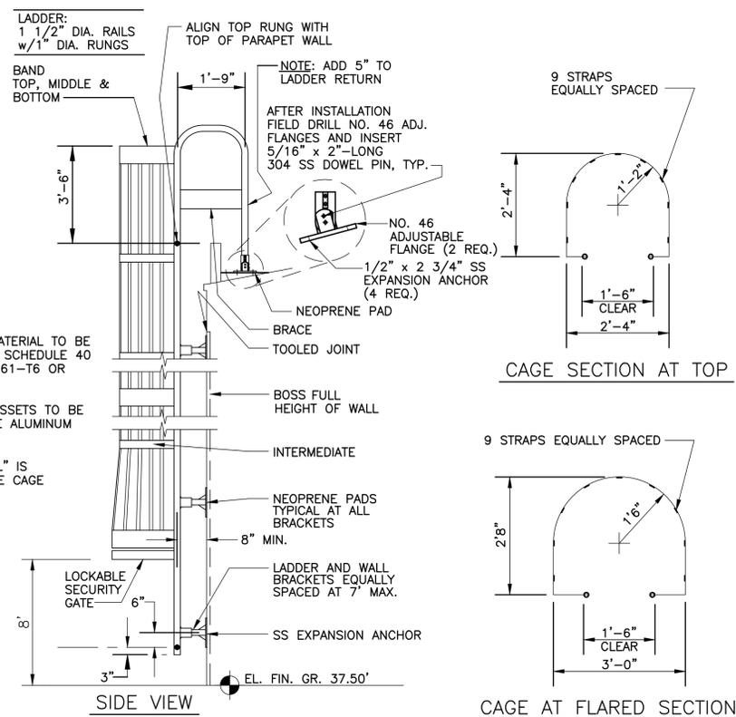
**EXTERIOR ALUMINUM LADDER WITH SAFETY RAIL, SAFETY CAGE AND LOCKABLE SECURITY GATE**
