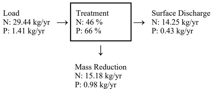
**Load Diagram for Multiple BMP ( As Used In Routing)**
