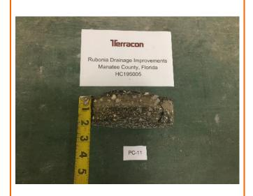
Core PC-11, 1 3/4" Asphalt (Full-Depth Crack)
