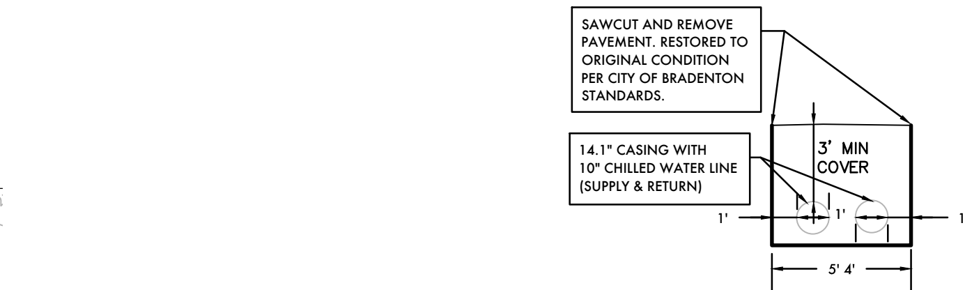
TYPICAL SECTION FOR TRENCHING & PIPE LAYOUT : STA 3+70 TO STA 7+05
