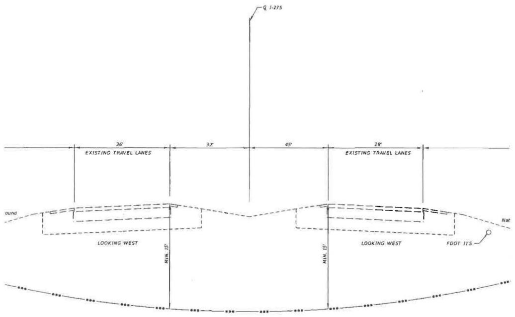
(1) 6" DIRECTIONAL BORE WITH TWO (2) 2" CONDUITS (HDPE) 6" PULL BACK REMER. MIN. DEPTH 180" OR 15 FT. DEEP
