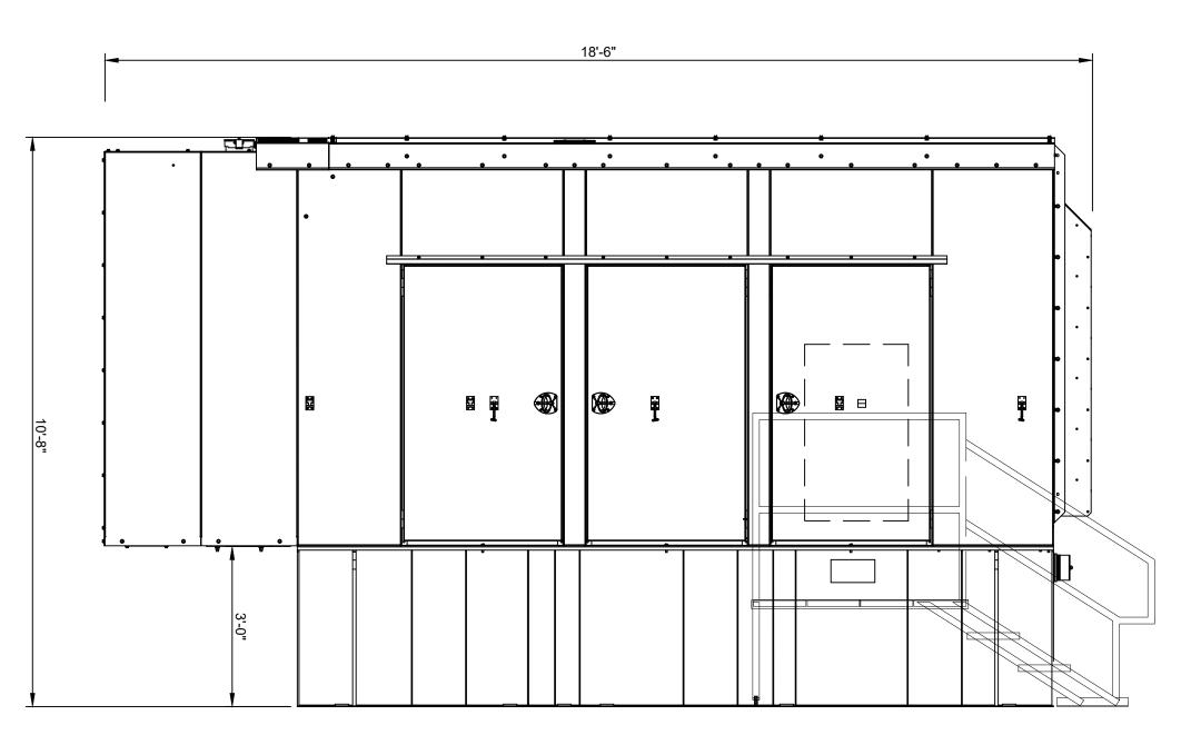
GENERATOR ELEVATION VIEW SCALE: 1/2" = 1'-0"
