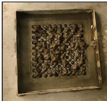
**SP test showing heavy extrusion**
