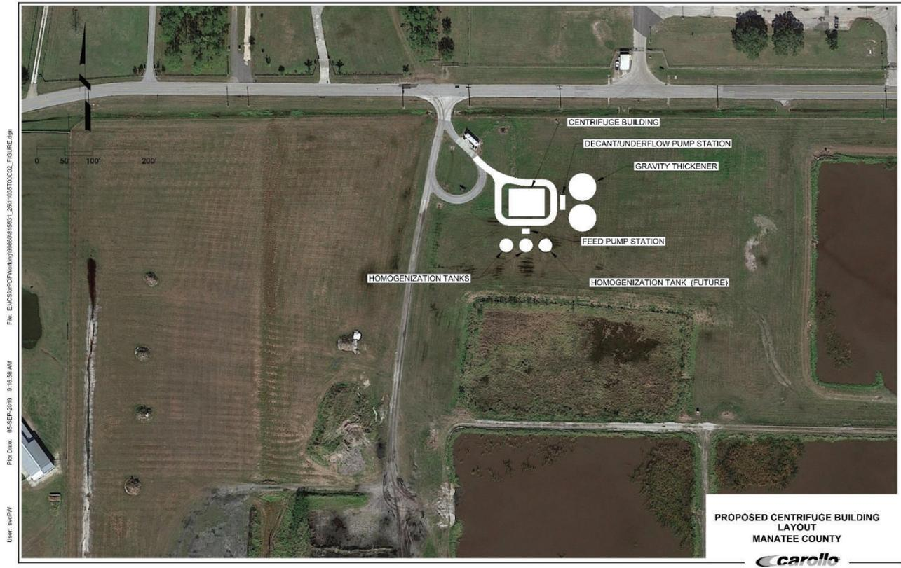
Figure 16 Centrifuge Facilities Layout
