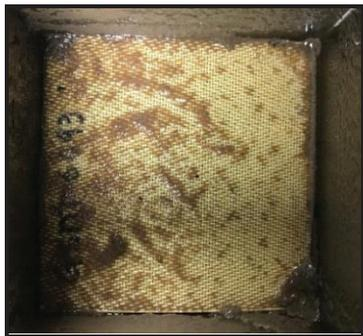
**Extrusion through Belt Filter**
