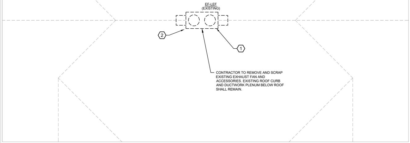
**1 MECHANICAL DEMOLITION PLAN: ROOF**
