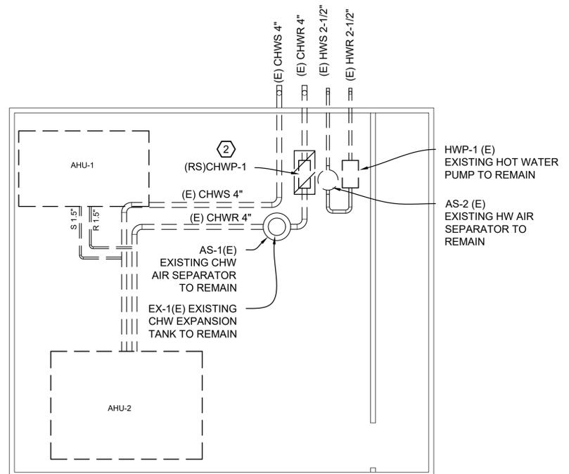
1 MECHANICAL ROOM DEMOLITION PLAN
