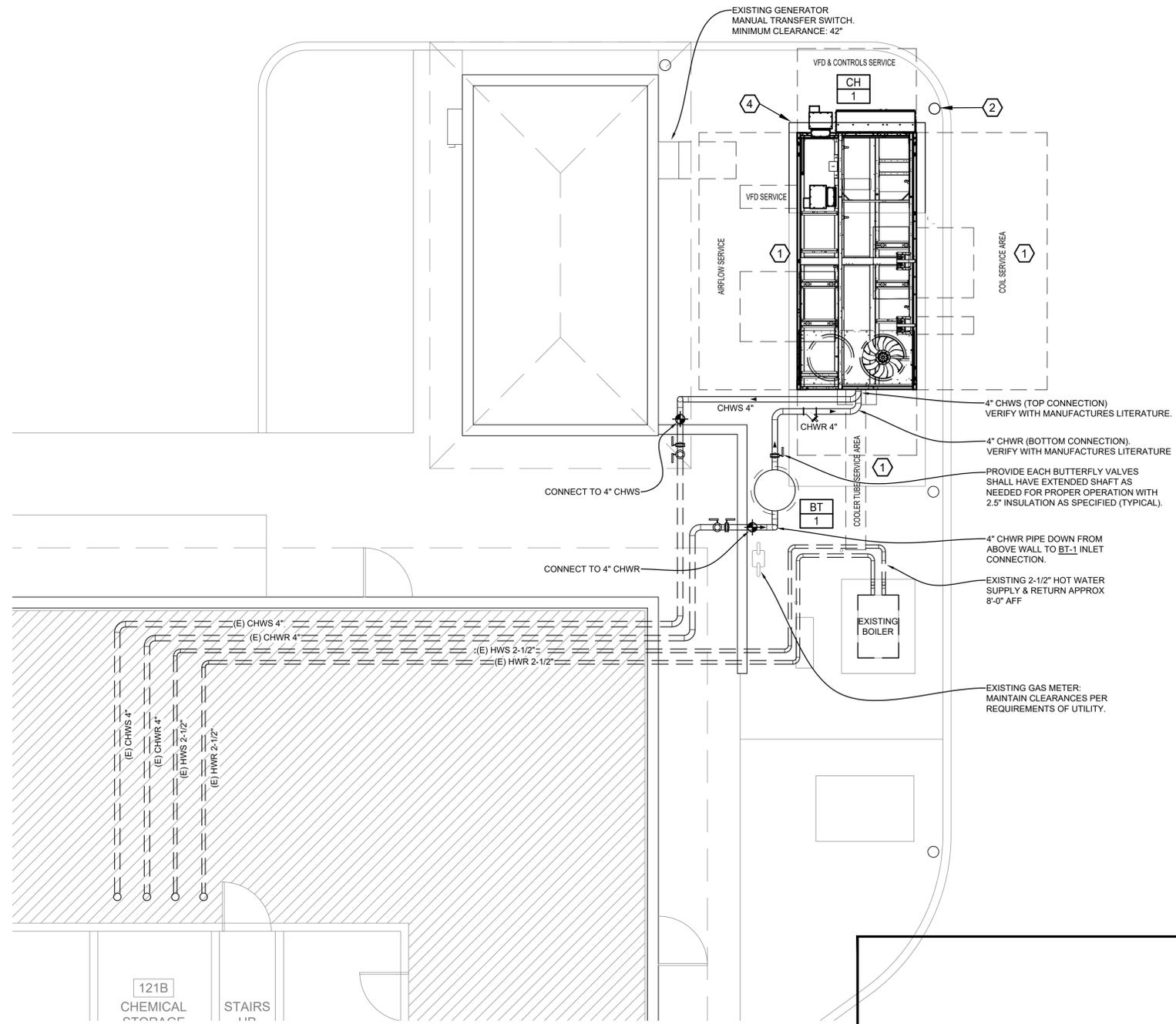
**2 MECHANICAL RENOVATION PIPING PLAN**
