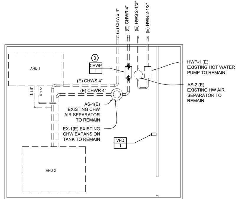
**1 MECHANICAL ROOM RENOVATION PIPING PLAN**
