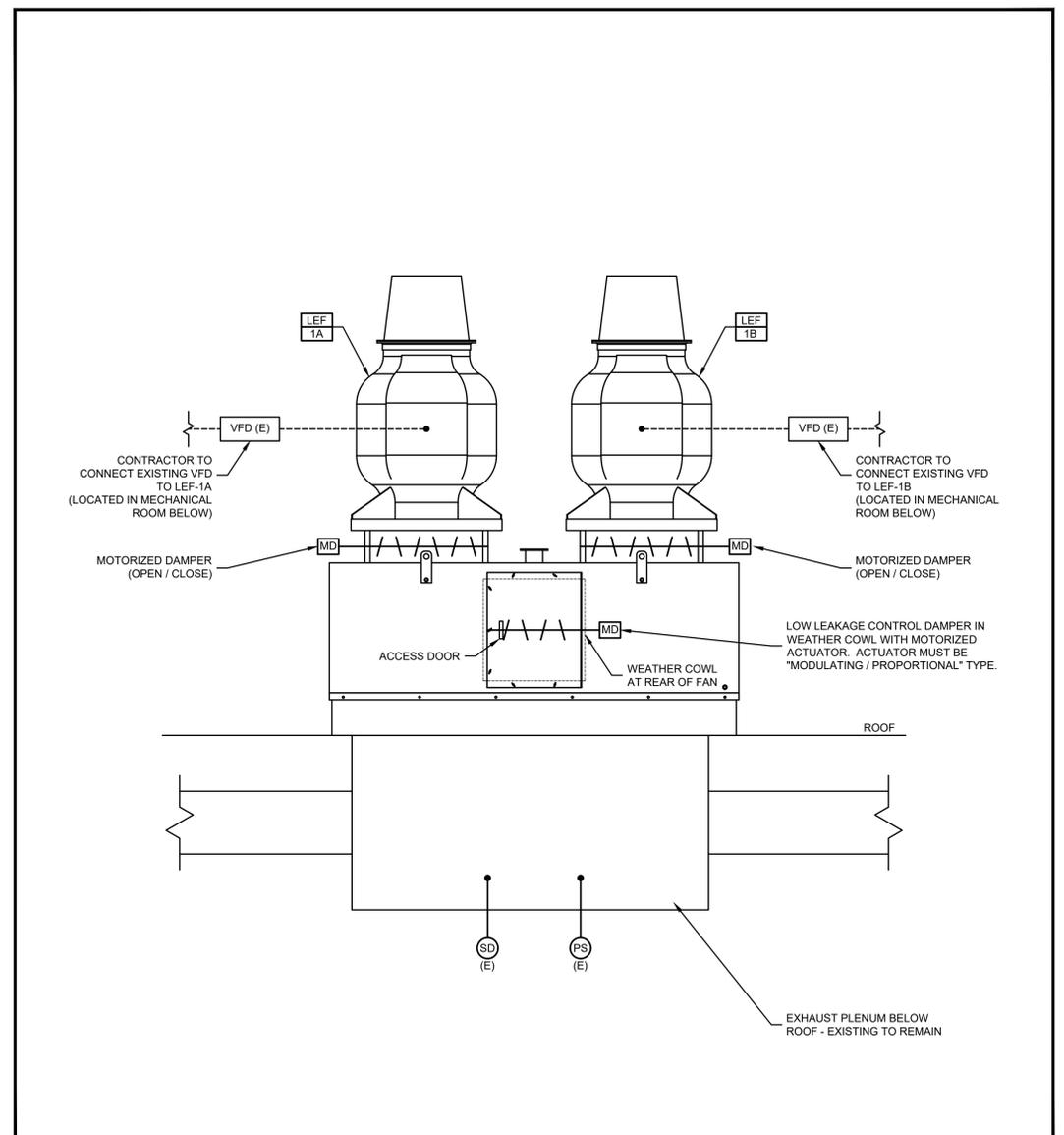
1 CONTROLS SCHEMATIC: EXHAUST SYSTEM
