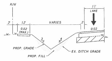
Figure 5 – Roadside Ditch
