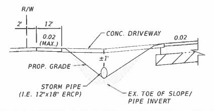
Figure 6 - Side Drain Cover
