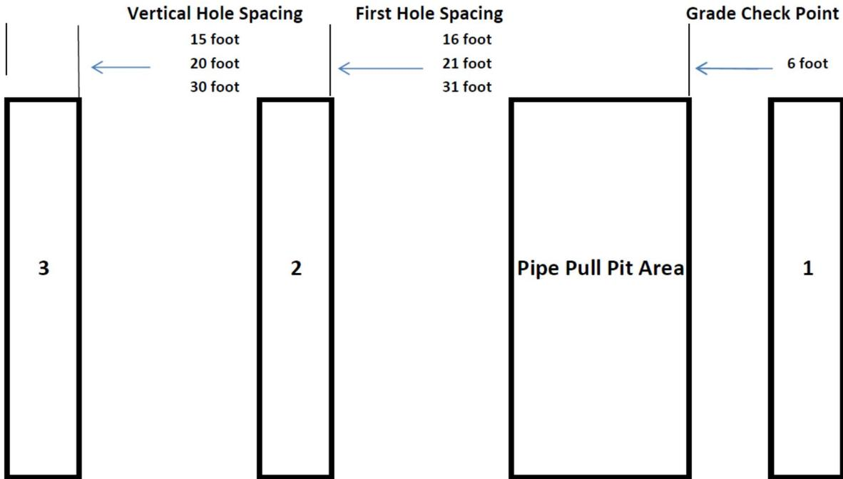
Pilot bore stem placement and stability. To the satisfaction of the Owner/Engineer, the contractor must use CTHDD approved tooling that will provide a method to control the pilot bore stem in the correct alignment prior to back reaming.
