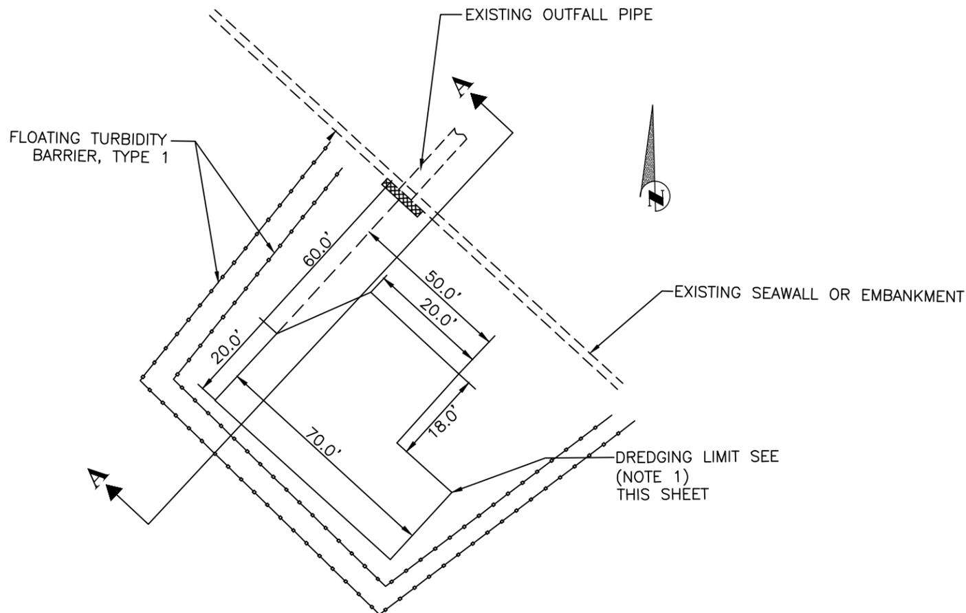
NOTE 1: DREDGING LIMITS NOT TO EXCEED AREA AS SHOWN AND TO REMAIN WITHIN PREVIOUSLY DREDGED AREA. MAINTAIN 10 FT MINIMUM SEPARATION FROM MANGROVES, DOCKS, SEAWALLS, AND OTHER MANMADE STRUCTURES
