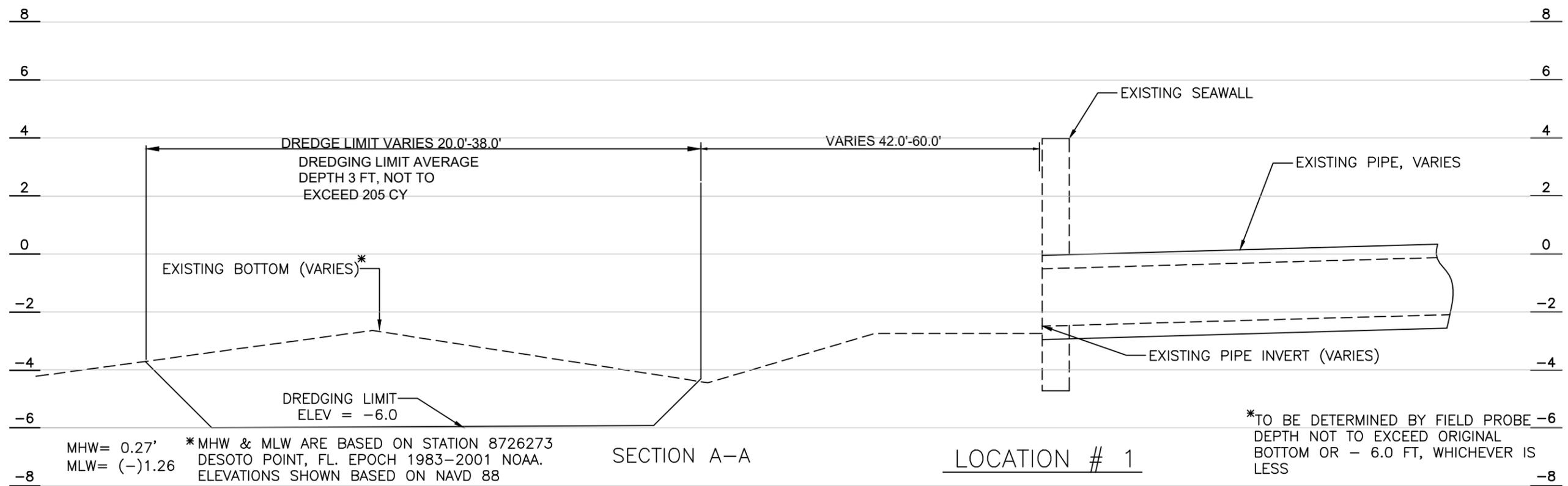
MHW = 0.27' MLW = (-)1.26 \*MHW & MLW ARE BASED ON STATION 8726273 DESOTO POINT, FL. EPOCH 1983-2001 NOAA. ELEVATIONS SHOWN BASED ON NAVD 88
