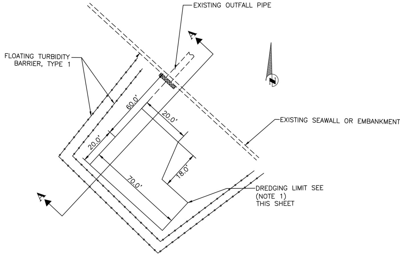
NOTE 1: DREDGING LIMITS NOT TO EXCEED AREA AS SHOW AND TO REMAIN WITHIN PREVIOUSLY DREDGED AREA. MAINTAIN 10 FT MINIMUM SEPARATION FROM DOCKS AND OTHER MANMADE STRUCTURES
