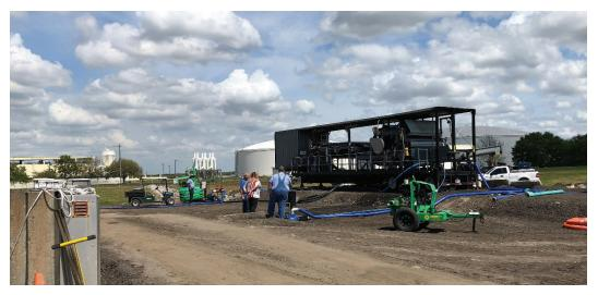
Figure 1 Temporary Belt Filter Press
