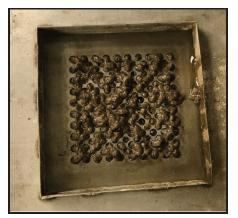
SP test showing heavy extrusion
