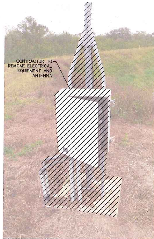
EX. EAST LAKE ELECTRICAL EQUIPMENT
