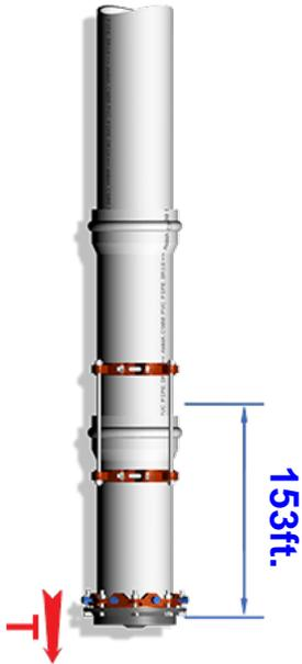
ALL JOINTS WITHIN THE CALCULATED LENGTH MUST BE RESTRAINED
