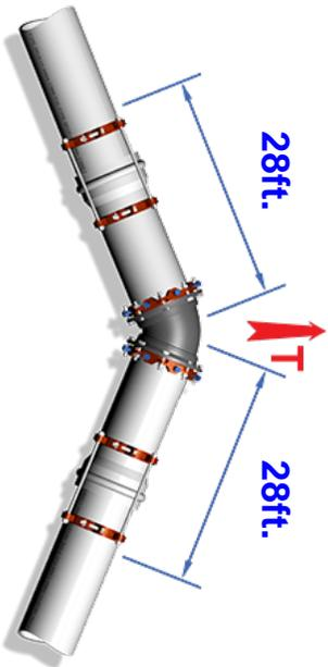
ALL JOINTS WITHIN THE CALCULATED LENGTH MUST BE RESTRAINED
