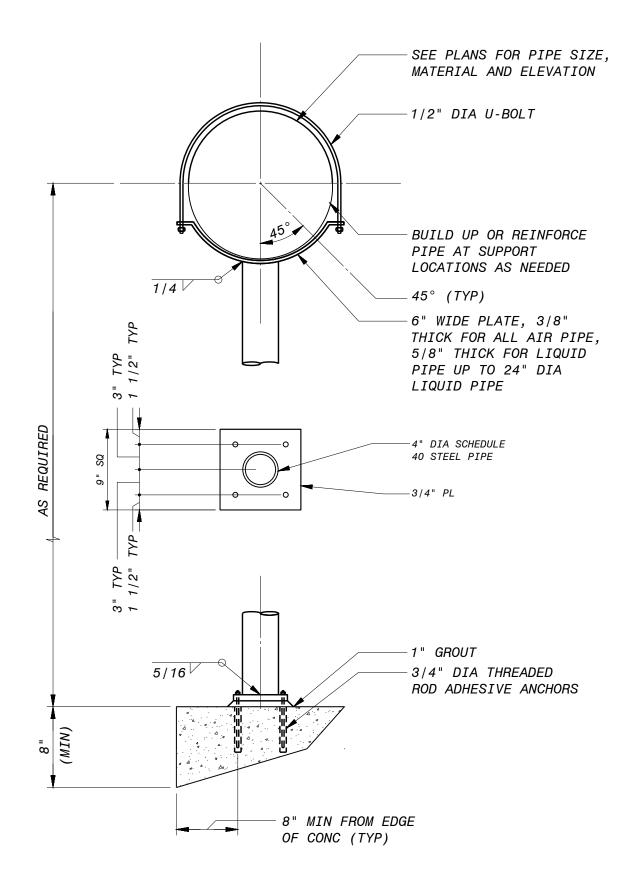
1. ALL STEEL MATERIALS SHALL BE HOT-DIP GALVANIZED FOR EXTERIOR LOCATIONS. VENT HOLES FOR GALVANIZING SHALL BE THE MINIMUM SIZE NECESSARY. HOLES SHALL BE LOCATED IN THE BOTTOM BASEPLATE AND ALSO LOCATED IN THE TOP OF THE PIPE, ADJACENT TO THE CURVED PLATE.
