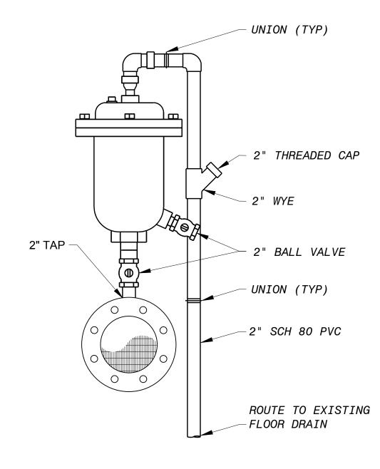
AIR RELIEF VALVE M-01 NO SCALE
