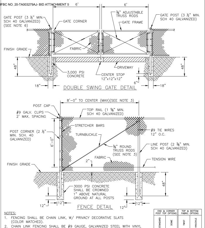
2. CHAIN LINK FENCING SHALL BE #9 GAUGE, GALVANIZED STEEL WITH VINYL COATING (BLACK OR GREEN).
