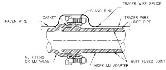
NOTE: SCHEMATIC SHOWN FOR STANDARD MJ FITTINGS AND GATE VALVES.
