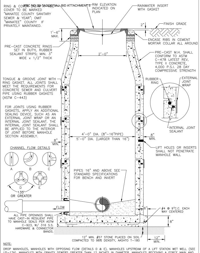
DROP MANHOLES, MANHOLES WITH OPPOSING FLOW (DETAILS D & E), MANHOLES UPSTREAM OF A LIFT STATION WET WELL (SEE US-17A), MANHOLES WITH GRAVITY SEWERS GREATER THAN 12 INCHES IN DIAMETER, MANHOLES RECEIVING A FORCE MAIN AND THE FIRST TWO GRAVITY MANHOLES DOWNSTREAM OF MANHOLES RECEIVING A FORCE MAIN SHALL BE A POLYMER CONCRETE MANHOLE (SEE US-3); OR EXISTING PORTLAND CONCRETE MANHOLE SHALL RECEIVE AN APPROVED LINER.
