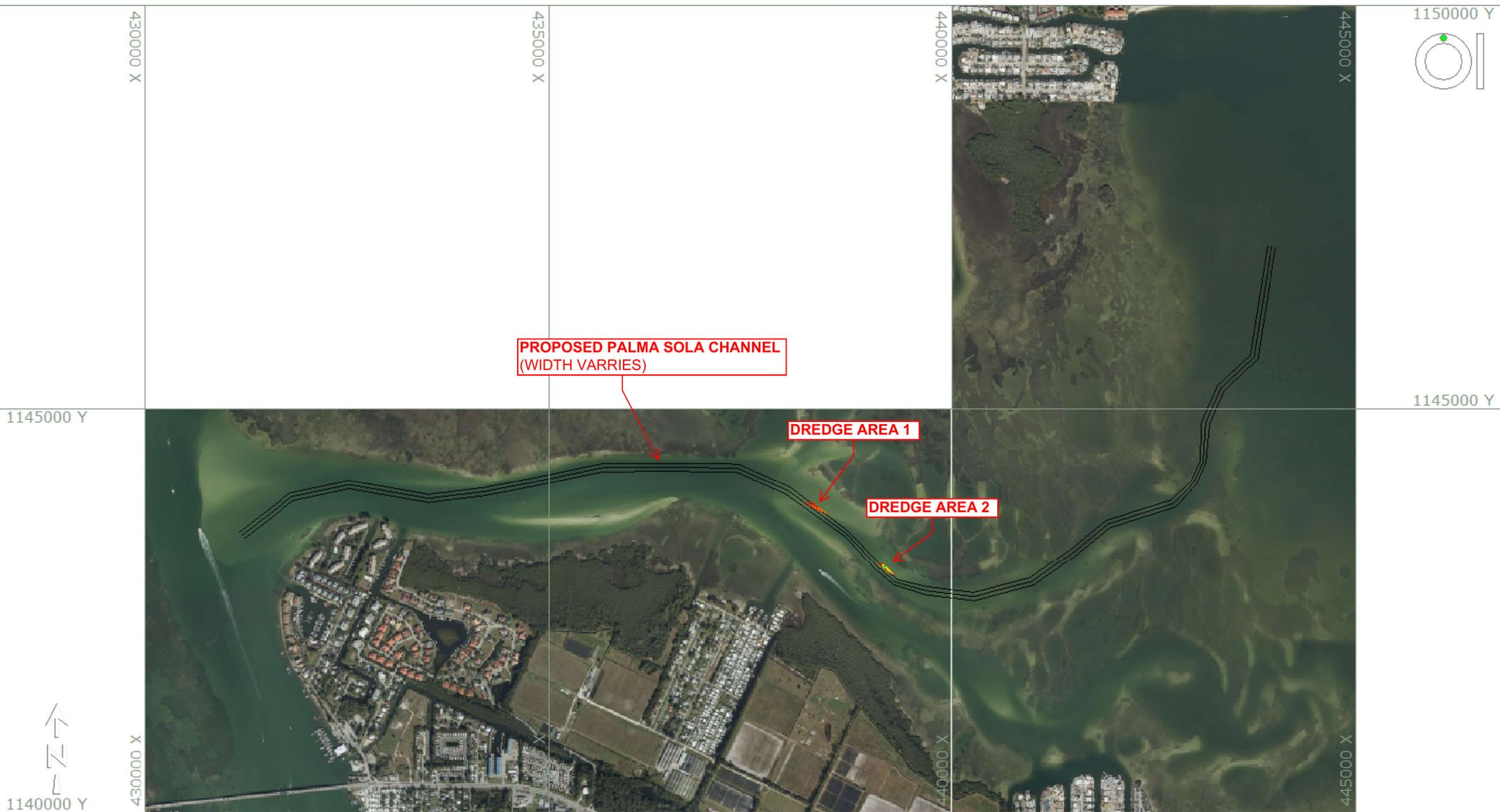
**FIGURE 5 - SURVEYED AREAS WITHIN OR NEAR PROPOSED CHANNEL WITH DEPTHS LESS THAN 4' MLLW**
