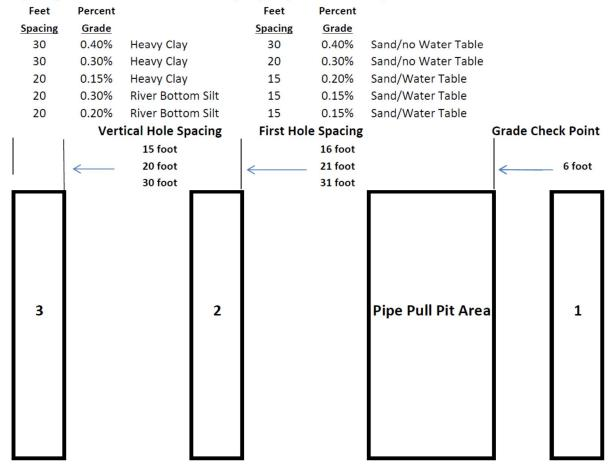
Pilot bore stem placement and stability. To the satisfaction of the Owner/Engineer, the contractor must use CTHDD approved tooling that will provide a method to control the pilot bore stem in the correct alignment prior to back reaming.
