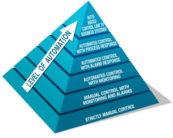
Figure 2.4 Level of Automation
