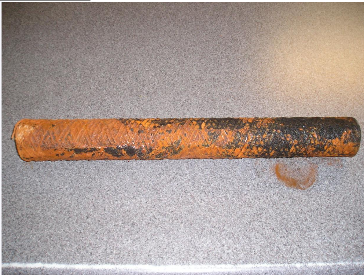
Figure 1: Digital photo of fouled cartridge filter.
