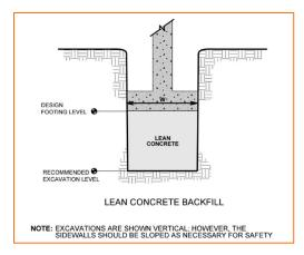
If unsuitable bearing soils are encountered at the base of the planned footing excavation, the excavation should be extended deeper to suitable soils, and the footings could bear directly on these soils at the lower level or on lean concrete backfill placed in the excavations. This is illustrated on the sketch above.
