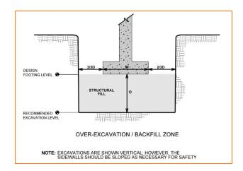
Over- excavation for structural fill placement below footings should be conducted as shown above. The over-excavation should be backfilled up to the footing base elevation with Structural Fill (as previously described) placed as recommended in the **Earthwork** section or FDOT No. 57 that is wrapped on all sides with a filter fabric and tamped.
