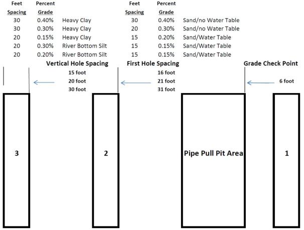
Pilot bore stem placement and stability. To the satisfaction of the Owner/Engineer, the contractor must use CTHDD approved tooling that will provide a method to control the pilot bore stem in the correct alignment prior to back reaming.
