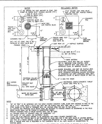
EXISTING MAINS. CONCRETE THRUST BLOCK IS ALSO REQUIRED UNLESS RESTRAINED JOINT LENGTH IS TREATED AS A PLUG SHOWN IN STANDARD DETAIL UG-8
