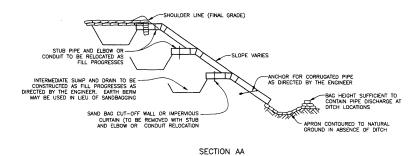
TEMPORARY SLOPE DRAIN FIGURE 15
