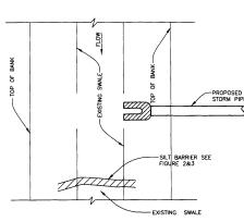
TURBIDITY BARRIER AT CONNECTION OF STORM PIPE TO EXISTING LAKE
