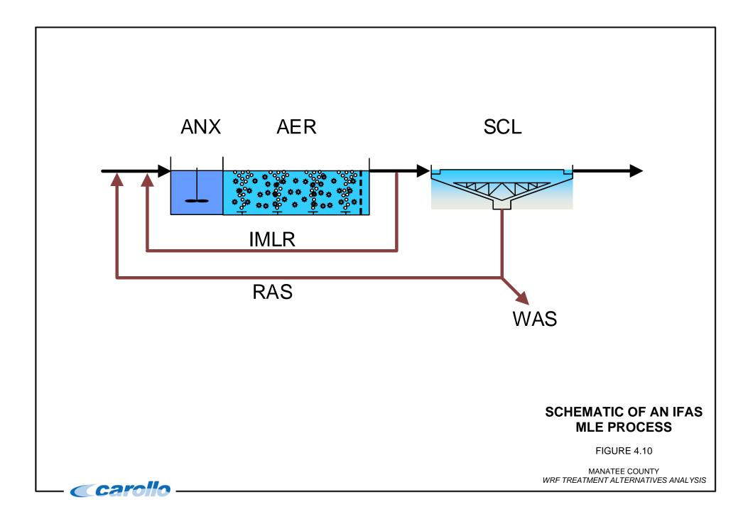
The advantage of an IFAS retrofit is that a relatively high culture of biomass may be maintained in the aeration basin to allow for a considerable increase in loading capacity. Since the increase is due to the fixed-film culture, there is not a significant increase in solids loading to the downstream clarifiers.
