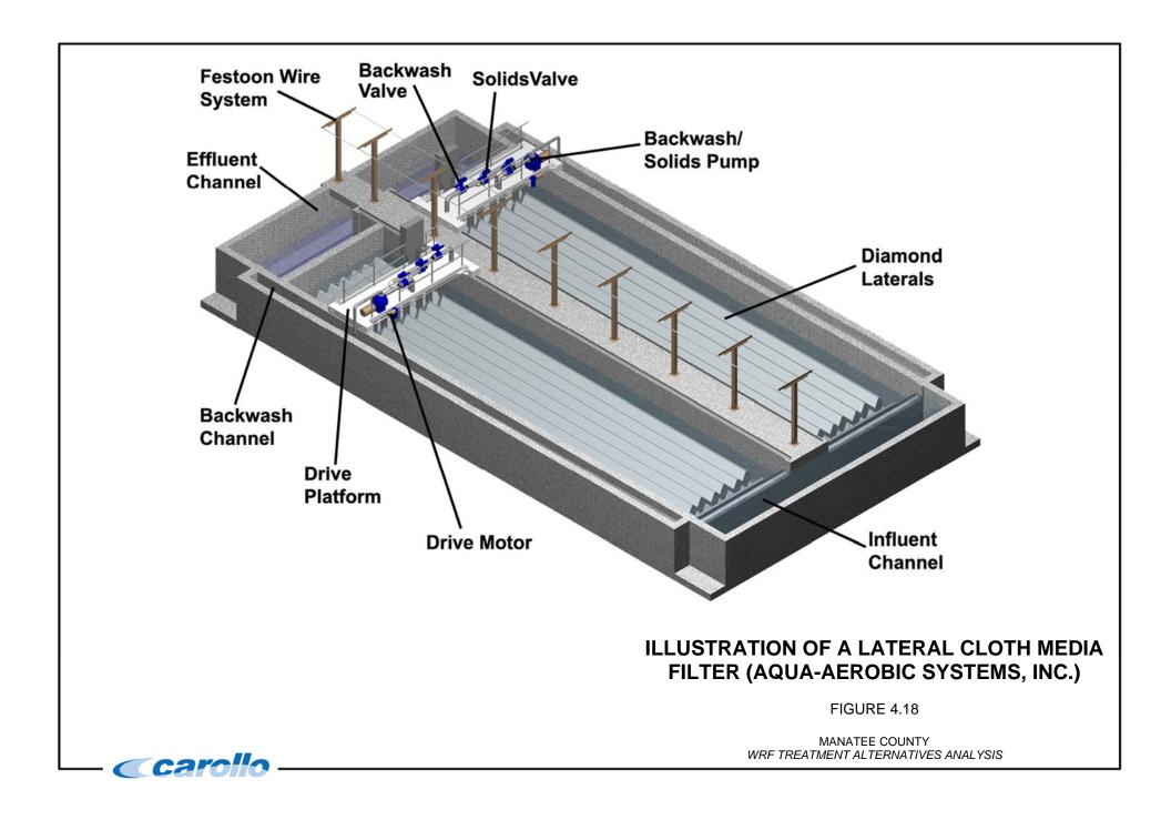
Performance of the various CMF designs varies by pore size of individual units, which can be had anywhere from 5 to 40 µm. Hydraulic throughput also varies by design. California Department of Public Health throughput limits on various CMF units ranges from 6 to 16 gpm/ft<sup>2</sup>. Most CMF designs including the disk layout typically require a custom design basin, but the lateral types can be retrofitted into an existing media filter tank with a long, narrow geometry.
