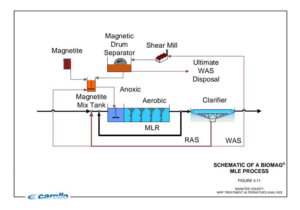
Secondly, magnetite is a magnetic compound so it has extremely high recovery rates using relatively low maintenance hammer mill/magnetic drum separator equipment on the WAS line.
