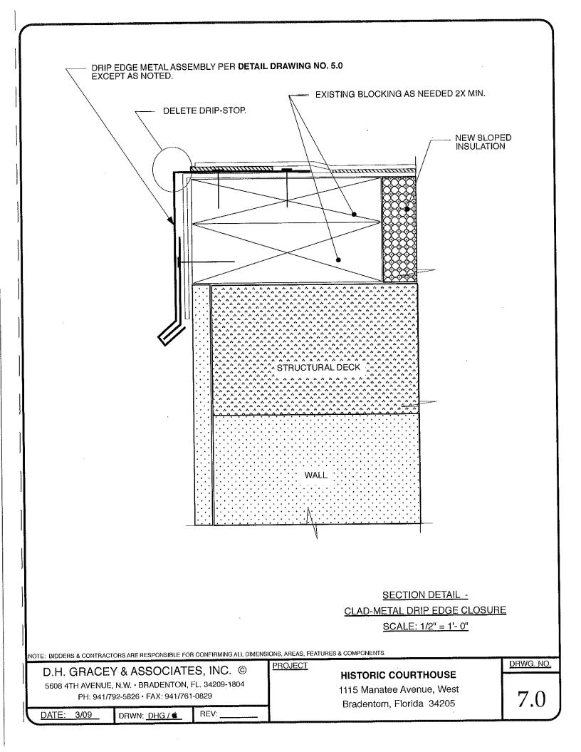
REFER TO DETAIL DRAWING NO. 4.0. FOR WALL TREATMENT. REFER TO DETAIL DRAWING NO. 7.0 FOR DRIP EDGE DETAIL. NOTE: BIDDERS & CONTRACTORS ARE RESPONSIBLE FOR CONFIRMING ALL DIMENSIONS, AREAS, FEATURES & COMPONENTS. PROJECT DRWG. NO. D.H. GRACEY & ASSOCIATES, INC. © **HISTORIC COURTHOUSE** 5608 4TH AVENUE, N.W. • BRADENTON, FL. 34209-1804 1115 Manatee Avenue, West PH: 941/792-5826 • FAX: 941/761-0829 8.0 Bradentom, Florida 34205 DATE: 3/09 REV: DRWN: DHG / #
