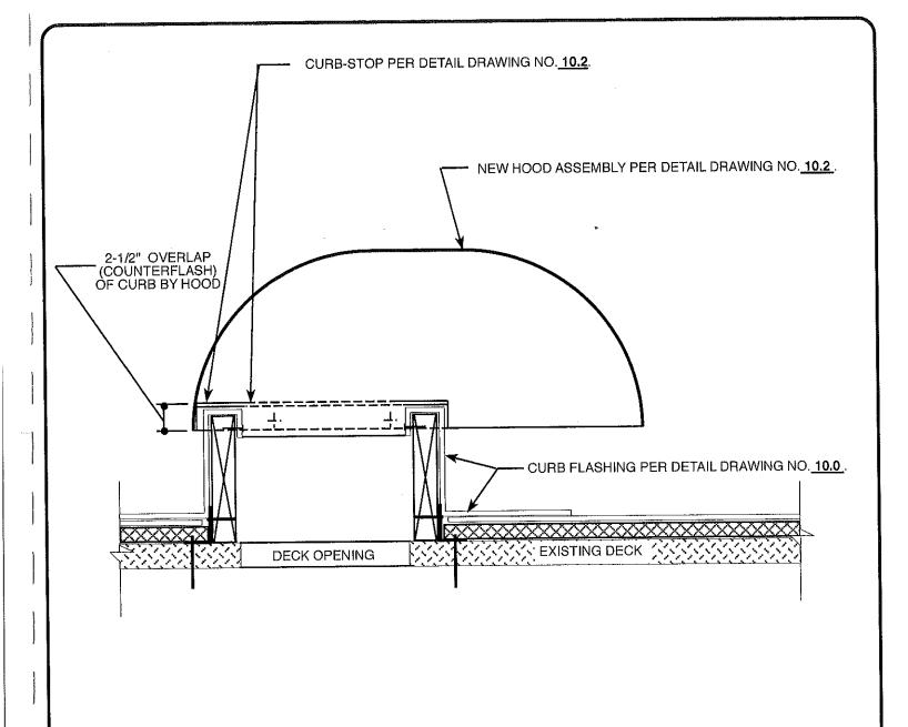
NOTE: REFER TO DETAIL DRAWINGS NO'S. 10.0 & 10.2 FOR CURB & HOOD FABRICATION.
