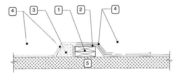
SECTION DETAIL TEMPORARY NIGHT SEAL
