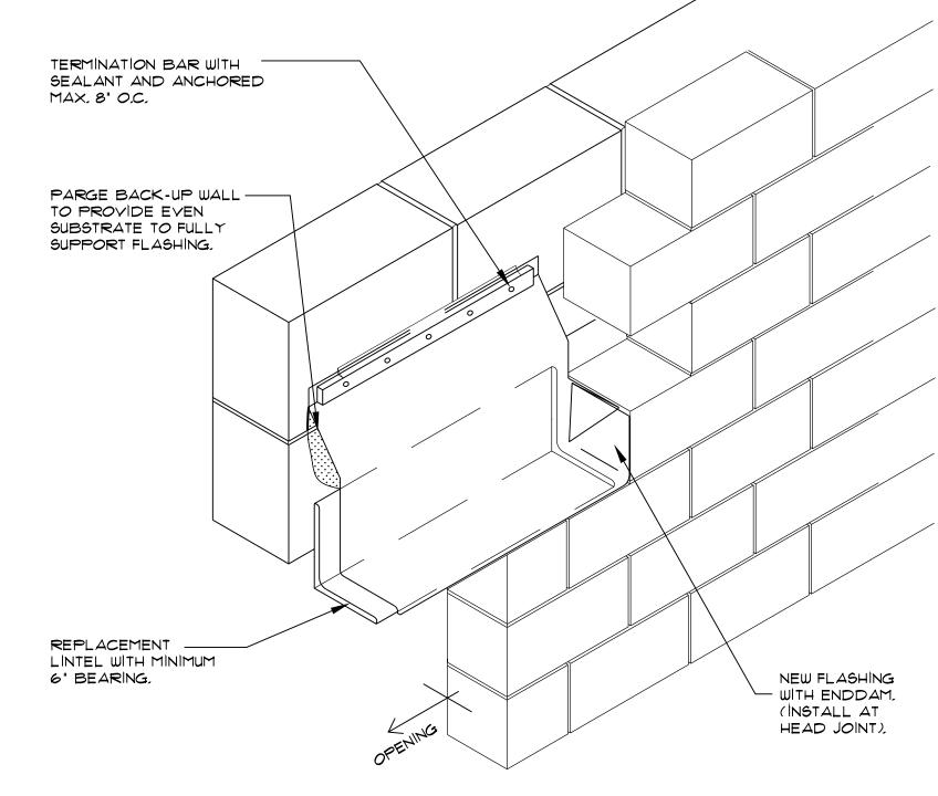
LINTEL AND FLASHING 3 REPLACEMENT DETAIL
