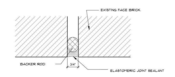
**PROPOSED VERTICAL JOINT** SCALE: 1 1/2" = 1'-0"
