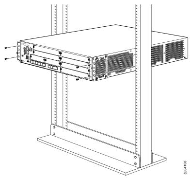
7. Verify that the mounting screws on one side of the rack are aligned with the mounting screws on the opposite side and that the services gateway is level.
