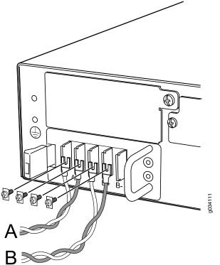
6. (Optional) If you have two DC power sources and wish to deploy A/B feed redundancy for the services gateway, connect the DC power cables to **B+** and **B-** terminals also.
