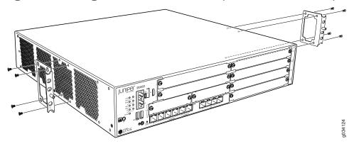
Figure 15: Installing the Rack Mount Brackets (Center Mount Position)
