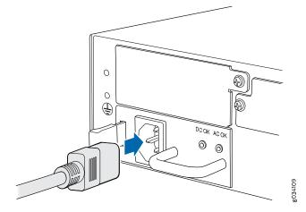
5. Dress the power cord appropriately. Verify that the power cord does not block the air exhaust and access to services gateway components or drape where people could trip on it.
