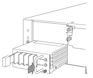
Figure 31: Installing a DC Power Supply on an SRX550 Services Gateway
