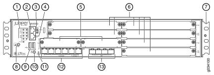
Figure 2: SRX550 Services Gateway Front Panel
