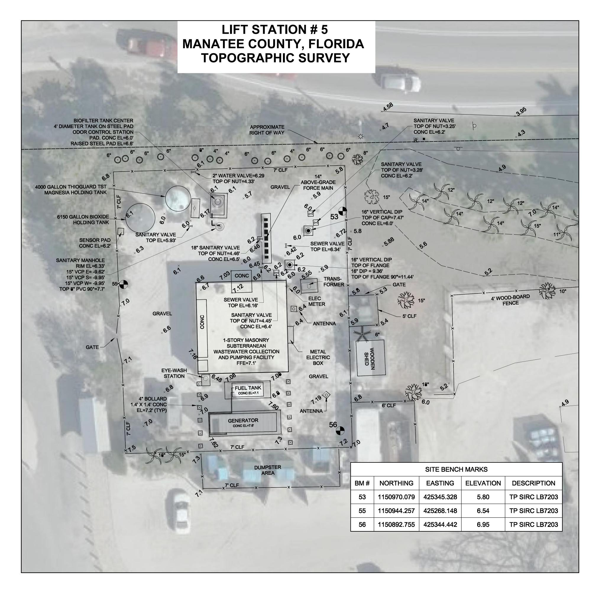
1. THE FOLLOWING NGS VERTICAL CONTROL MONUMENTS WERE RECOVERED AND UTILIZED FOR THE ELEVATIONS INDICATED HEREON: "J 254" PID AG1981 NAVD 1988 ELEVATION 13.48' AND "GIS 103" PID AG9208 NAVD 1988 ELEVATION 4.27"
