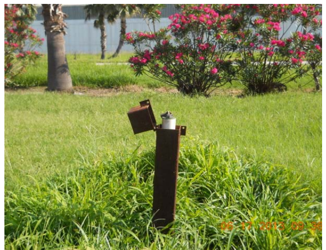
Site Photo 12: Stick-up monitoring well MW4-02.
