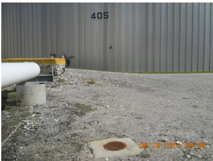
Site Photo 11: Flush-mount monitoring well MW5-02.
