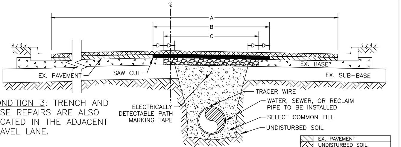
CONDITION 3: TRENCH AND BASE REPAIRS ARE ALSO LOCATED IN THE ADJACENT TRAVEL LANE.
