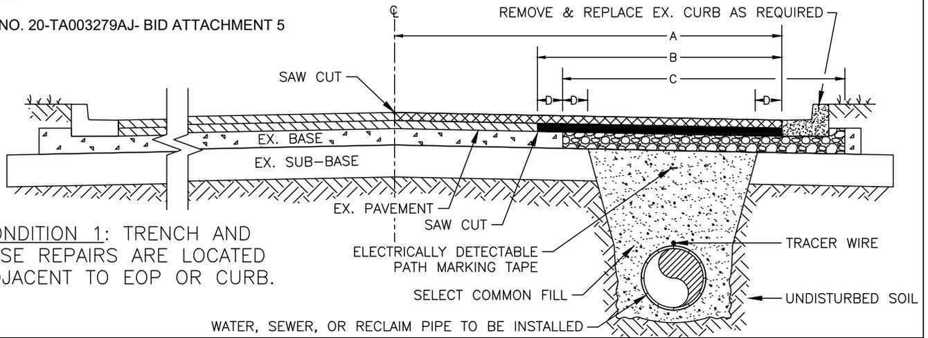
CONDITION 1: TRENCH AND BASE REPAIRS ARE LOCATED ADJACENT TO EOP OR CURB.
