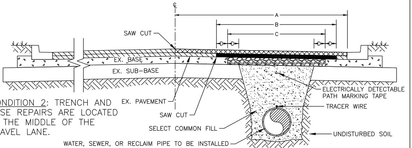
CONDITION 2: TRENCH AND BASE REPAIRS ARE LOCATED IN THE MIDDLE OF THE TRAVEL LANE.
