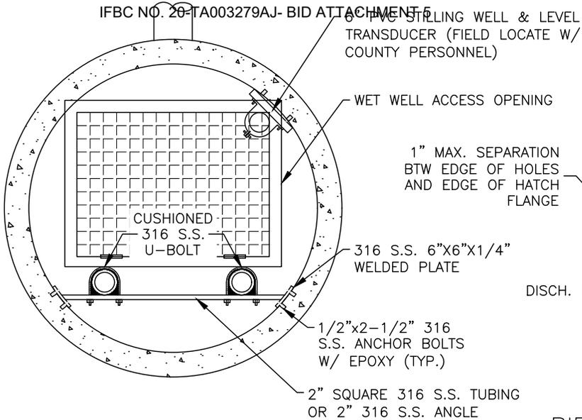
WET WELL PIPE BRACING DETAIL
