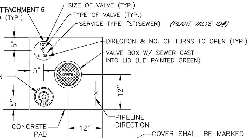
24"x 24"x 6" CONC. PAD TO BE INSTALLED AT EACH VALVE BOX.
