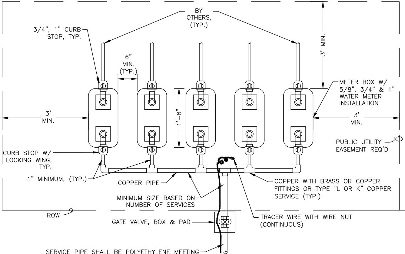
SERVICE PIPE SHALL BE POLYETHYLENE MEETING AWWA C-901 HDPE; OR TYPE ("K" OR "L") COPPER; OR STAINLESS STEEL SCHEDULE 40 PIPE. PIPE SHALL BE BLUE OR ENCASED IN A BLUE SLEEVE FOR POTABLE; PURPLE OR ENCASED IN A PURPLE SLEEVE FOR RECLAIMED WATER.
