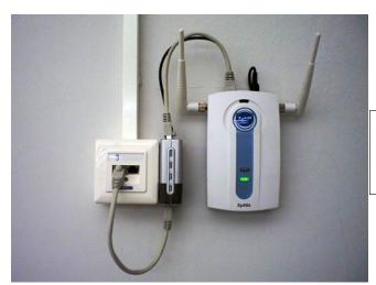
Given a single Power over Ethernet connection (single gray cable looping below), a PoE splitter provides both data (gray cable looping above) and power (black cable also looping above) connections for a wireless access point. The splitter is the silver and black box in the middle, between the wiring box on the left and the access point (with its two antennas) on the right. The PoE connection eliminates the need for a nearby power outlet.
